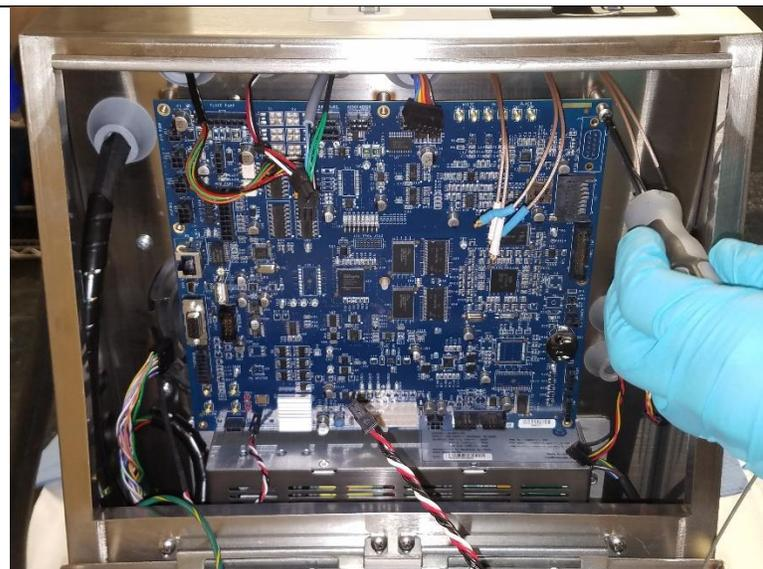
8. Connect the cables, then re-attach the door lanyard.
