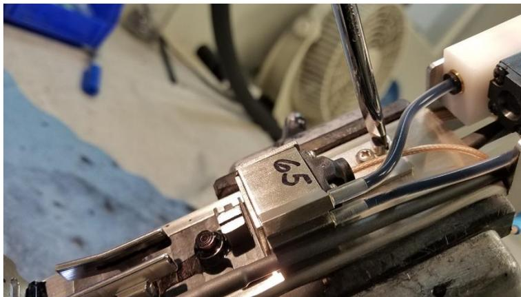
3. Tighten the drop generator adjuster screw once this position is achieved.
