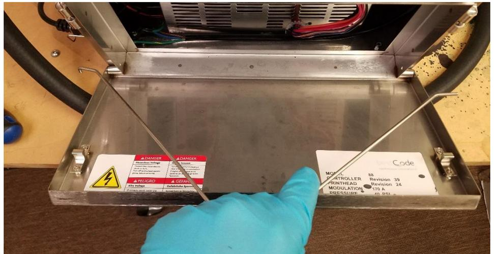
2. Insert the 46-5004-01 Filter, Air frame backing into the Air Filter box.
