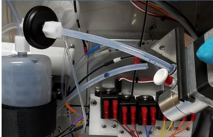
Red side fitting connects to the main ink filter tube (pump outlet).
