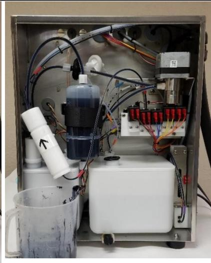
4. Remove the tube from the 1/8" push to connect PH Feed/Dampener filter output fitting.
