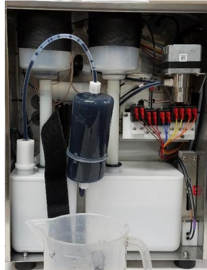
3. Place a wash beaker (47-0021-01) underneath the filter.
