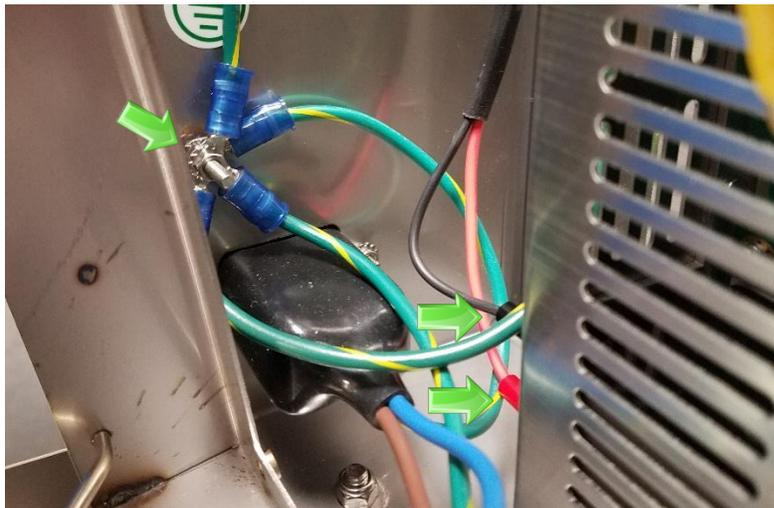
2. Pull the printhead harness forward to ensure all of the cables are disconnected from the Main CPU Board.
