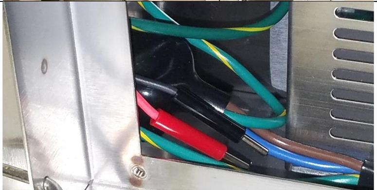
4. Remove the Main power entry cable from the power supply
