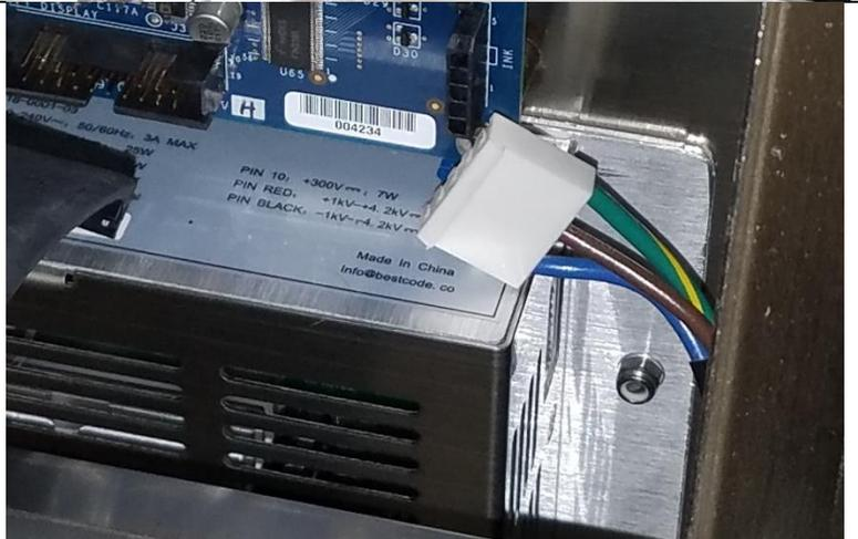
5. Remove the 7 M4 nuts that secure the power supply to the Controller Middle wall.
