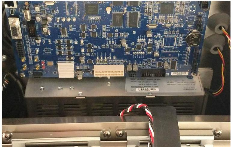
3. Remove the High Voltage jacks from the power supply
