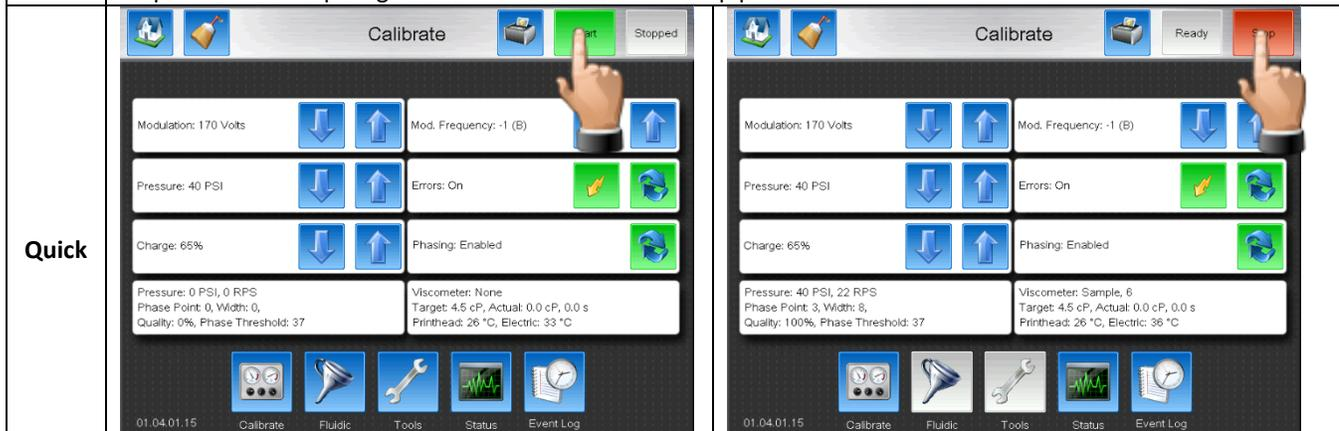
**Quick Start & Quick Stop** are technician tools to quickly start and stop the jet. They do not utilize makeup in the start, so they will not start or stop as clean as the Clean Start or Stop. The system will intelligently switch the Clean Start & Stop method to quick start to prevent the operator from adding too much makeup.
