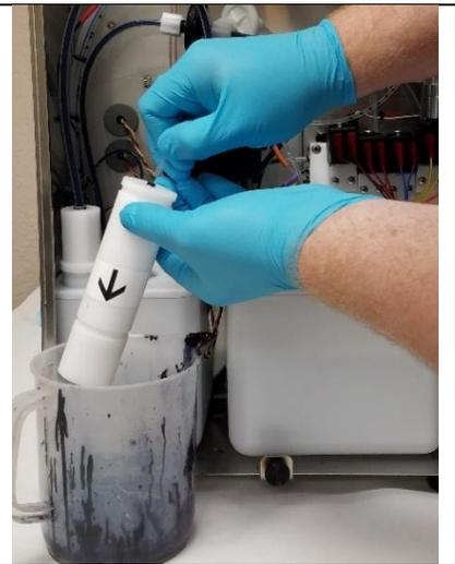
6. Install the new PH Feed/Dampener Filter in the same orientation as shown. The arrow be pointing in the direction of the ink flow.
