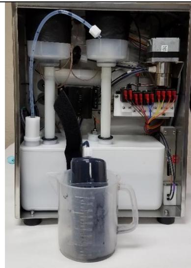
6. Loosen the compression nut on the filter input side. (use 5/8" open end wrench)
