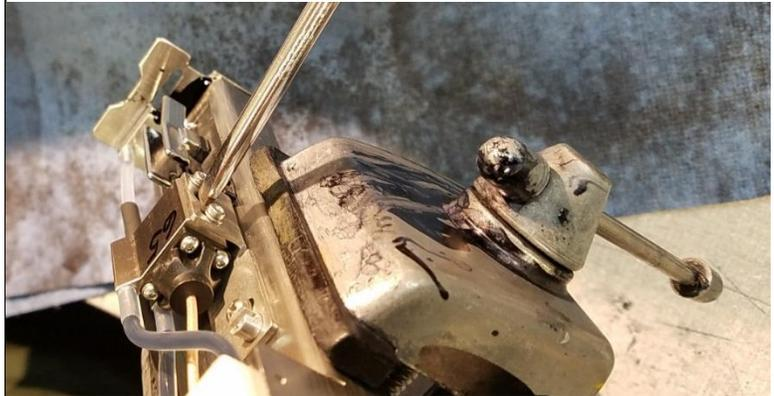
3. Tighten the 2 drop generator side mounting screws once this position is achieved.
