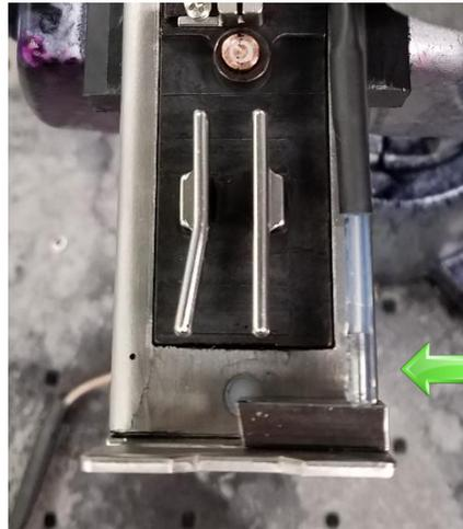
9. Apply the new heatshrink over the gutter detect and over the black coax cable connection.
