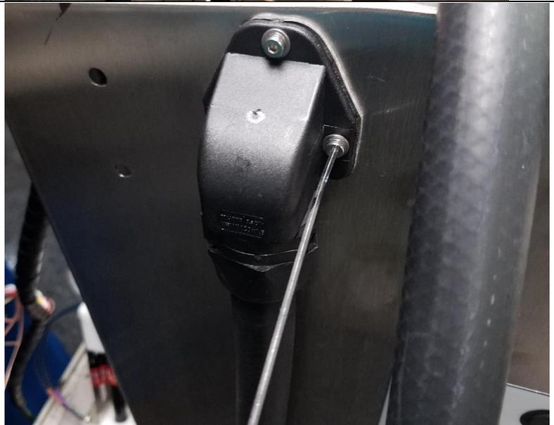
5. Lift out the Ink Manifold and remove the Blue, White, and Yellow tubes.
