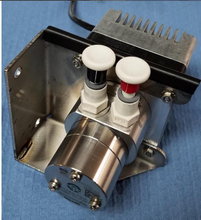
Pre-pump filter side connects to the black marked fitting (pump inlet).
